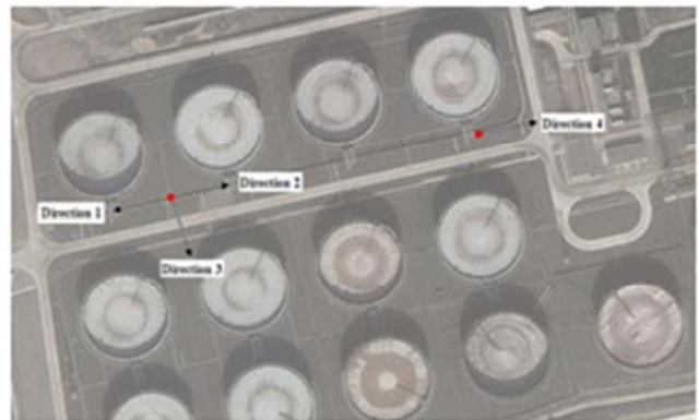
Figure 9. Potential gradient test direction.
